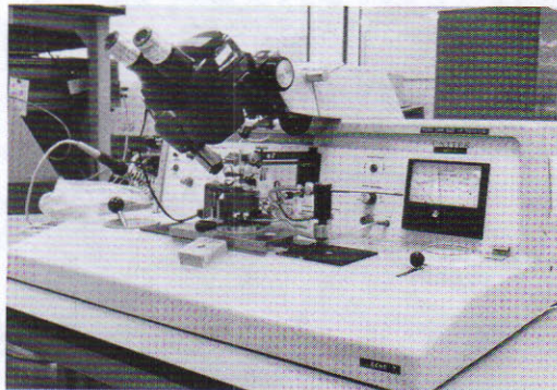
Figure 3. The Unitek Model 8-150-02 Bonder is Adaptable for the Thermocompression Bonding of Beam Lead Devices.
